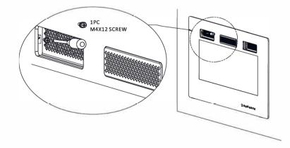
( Only for all models of style C which has no mesh for the air inlet . )
