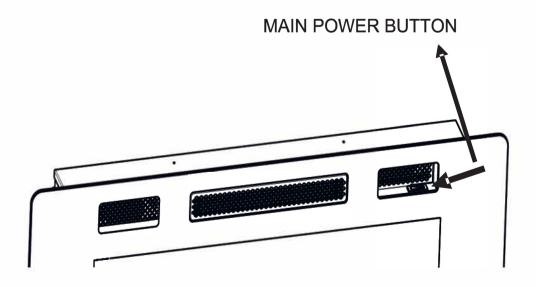
Note: Make sure the Main Power Switch is turned on before operating.
